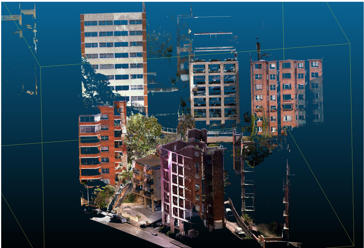
3d view of the 'point cloud' survey from TSS Total Surveying Solutions.
